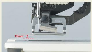
The work clamp foot height can be increased up to 12 mm, enabling the machine to make high-quality buttonholes in heavy-weight materials. The lifting of the work clamp is driven by a motor, which reduces operator work. The operation can be easily done with one pedal.
