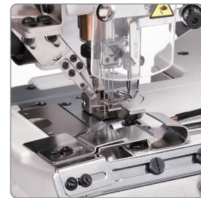
CY (CRL178-A) 氣動式環型鬆緊帶折縫 Pneumatic Tubular Elastic Tape Hemming
